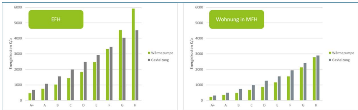
Figure 10: Comparison of heating costs for gas heating systems and heat pumps in 2022 for a detached house and a flat
