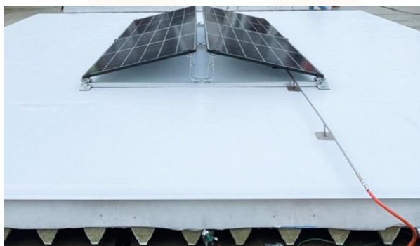
Figure 3: Tested PV system consisting of glass-foil modules in an east-west orientation.
