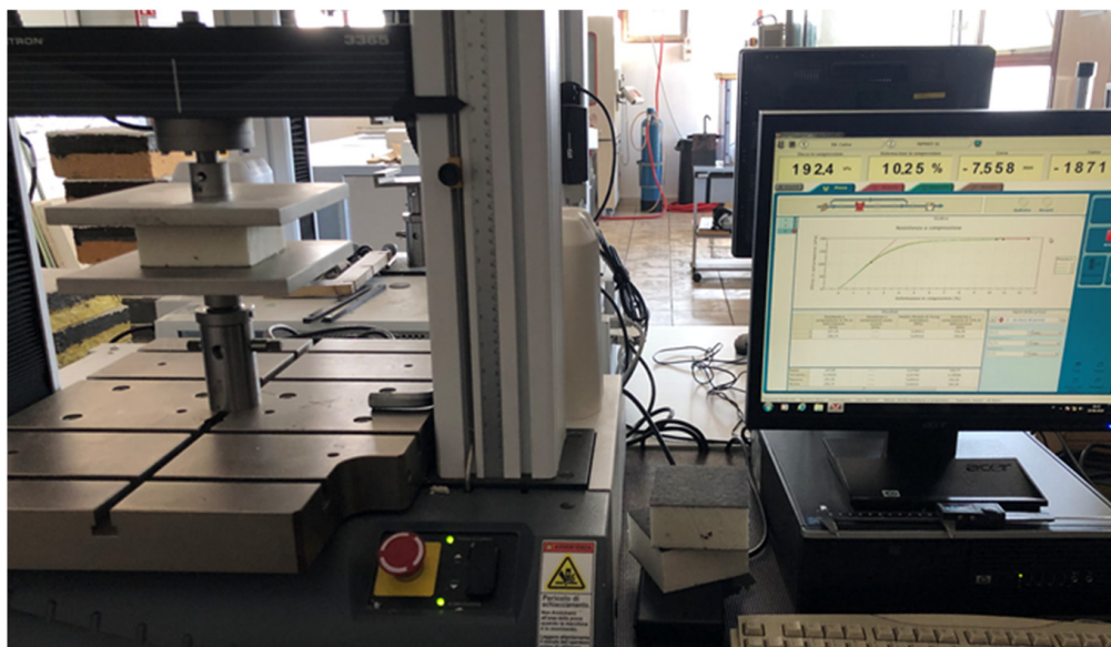
Figure 5. Compression test according to EN code 826; the machine apparatus is on the left and the report curve is on the right.
