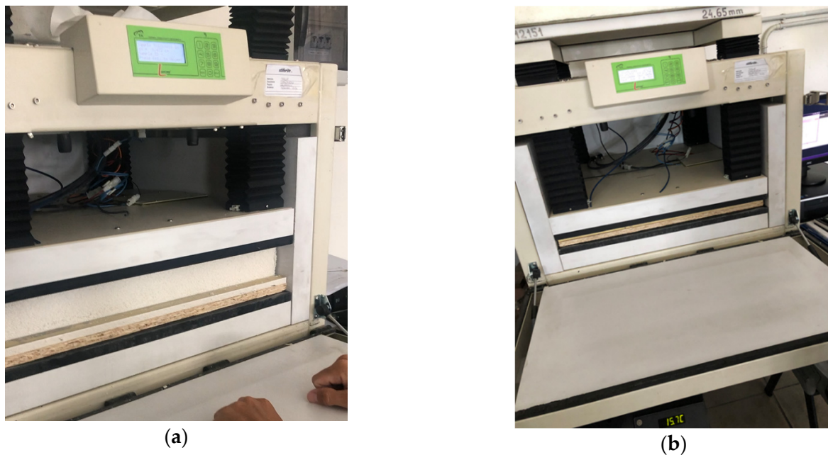
Figure 2. (a) Thermal resistance measurement according to EN 12667; (b) thermal resistance measurement of the stratigraphy needed to determine thermal resistance of each single material.
